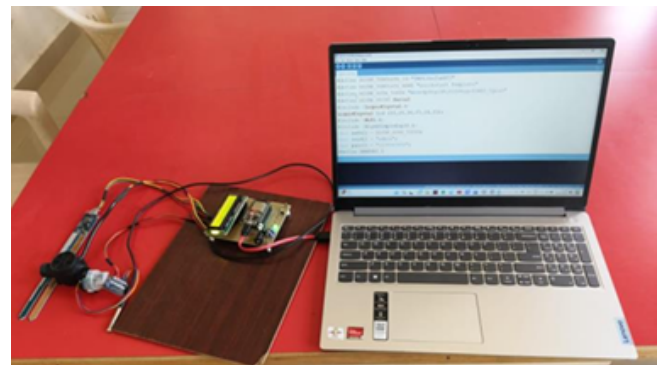
Fig.1 Connection of Sensors with Arduino UNO board and LCD display
