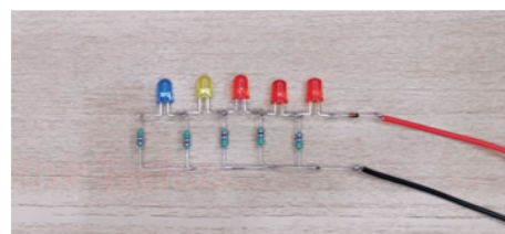
Figure 14. Indication of battery level using LED
