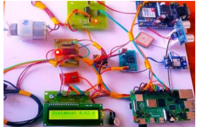
Figure.8 Ultrasonic Sensor Detects the Distance of The Object
