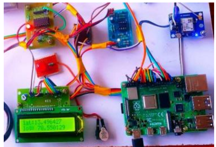
Figure. 9 Latitudes and Longitudes Are Identified Using GPS Receiver.
