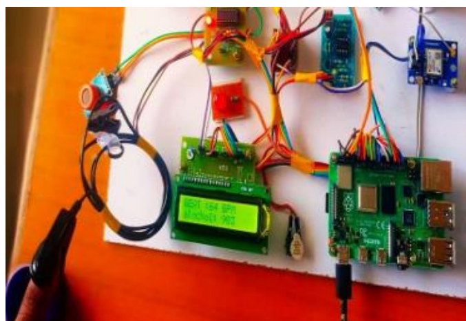
Figure. 8 Heart Beat Sensor Detected Heart Rate in BPM
