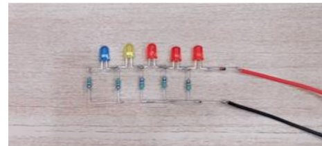
Figure 14. Indication of battery level using LED
